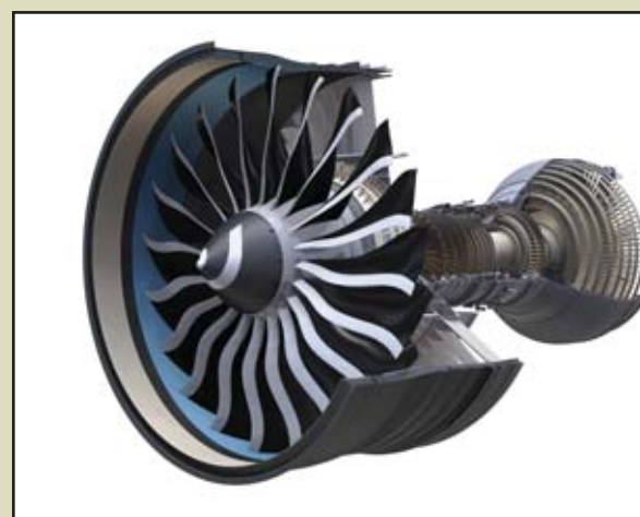
General Electric's GEnx powerplant offers a host of benefits over current-generation turbofan engines, thanks in part to composite components, which make the GEnx lighter than comparably sized engines.
