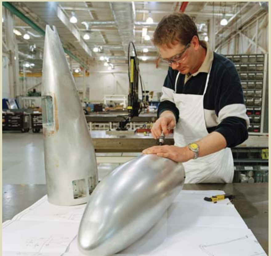
A Boeing employee works on the nose section of the 787 high-speed wind tunnel model, which has been used to confirm the advanced aerodynamic characteristics of the Dreamliner.
