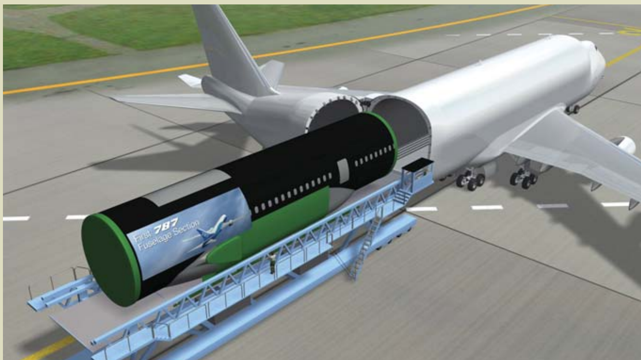
Boeing's new production system for the 787 will include air transport of many major assemblies via the Large Cargo Freighter, a modified 747-400F that will feature an aft fuselage that can swing open during loading and unloading operations.
